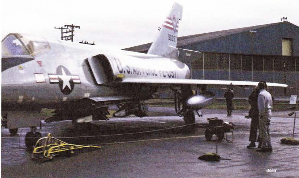
◀ Convair F-106 Delta Dart on display during an open house at Duluth AFB. Note missiles are extended position from the internal weapons bay.
