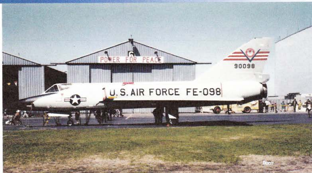
▲ Another F-106 on display during an open house at Duluth AFB. Note missiles are not visible, being carried in an internal weapons bay for clean supersonic flight.
