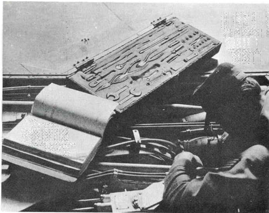
With this shadowbox kit, the mechanic can easily tell if he has left a tool where he shouldn't.
